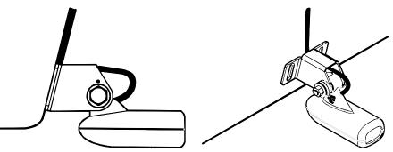
For single-frequency Skimmer, route cable over bolt and through bracket. Side view shown (left) and seen from above (right). **Both bracket types:** Attach the transducer to the transom. Slide the transducer up or down until it's aligned properly with the bottom of the hull as shown in the preceding and following figures. Tighten the bracket's mounting screws, sealing them with the caulking compound.
